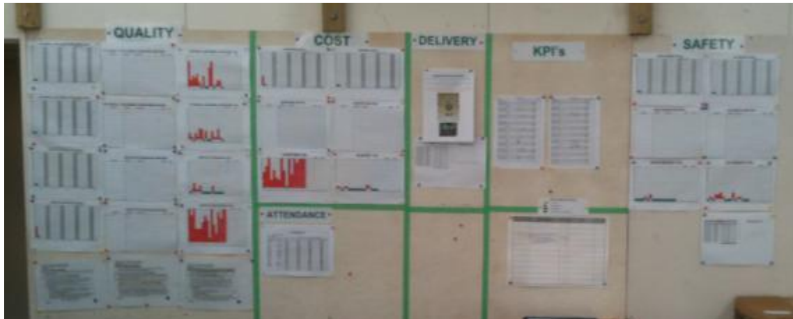
Figure 15: The nerve centre of every morning's Green Room meeting for delivery personnel, the visual management board
