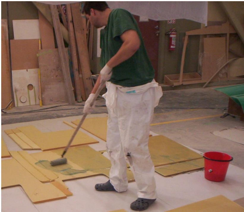
Figure 6: Improved application of resin on the foam through use of long handled roller reduces time and repetitive awkward movements.
