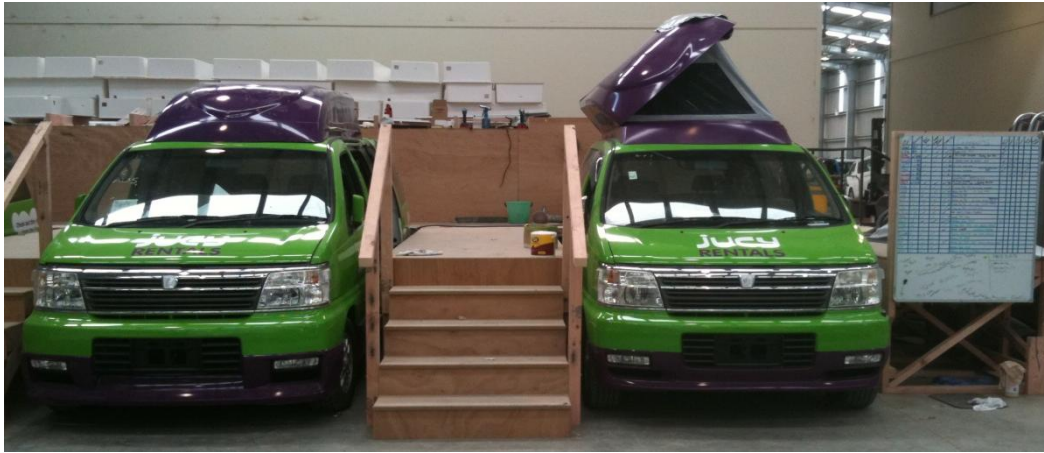
Figure 6: Mezzanine platforms make the installation of roof-top sleeping cabins easier and safer.
