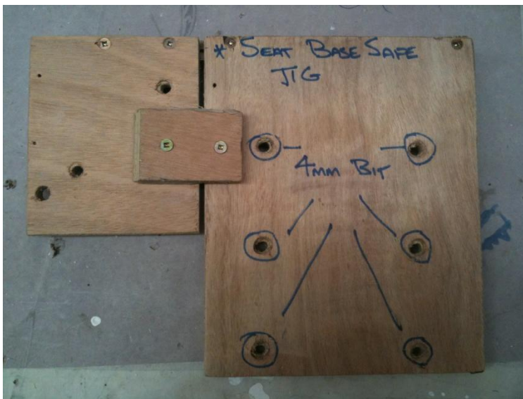
Figure 7: Sample jig helping to improve quality and delivery time
