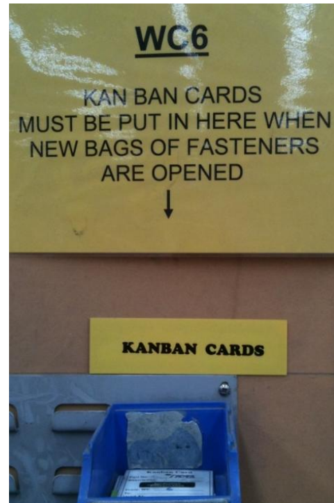
Figure 7: Kanban cards are placed into this bin and collected once a day by the store man for restocking.
