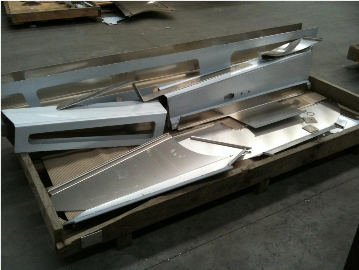
Figure 4: Kanban pallet; all components seen are for one specific boat. Each component carries an identification number linking it to a specific boat build.
