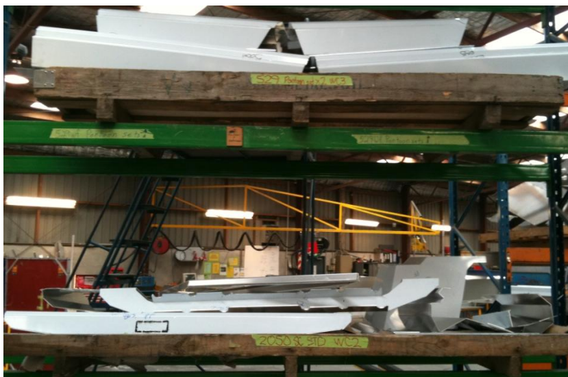
Figure 5: Kanban pallets containing components for specific boat builds. Identification numbers link each pallet to a specific build and work station.
